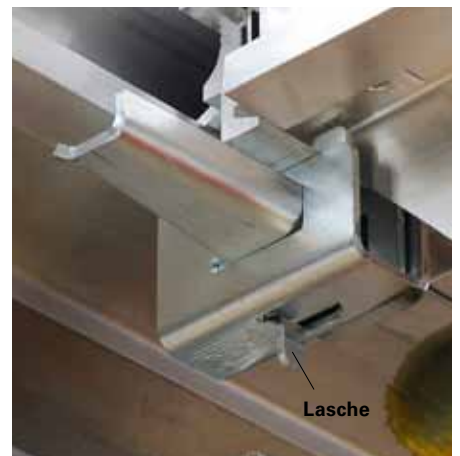
The lug of the Slab Coupler engages the opening of the slab prop and secures this against tipping over.
